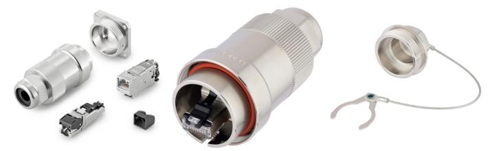
**Product features** Housing: brass nickel plated Qualified for 10 Gigabit/s Ethernet Suitable for stranded cores with AWG27/7 -22/7 and for solid conductors with AWG26/1- 22/1
