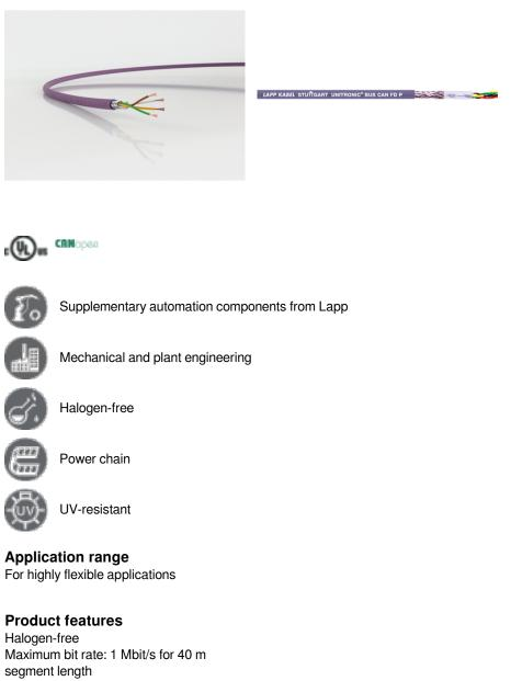
Larger conductor cross-section is necessary with increasing length. Refer to the table below (reference values from ISO 11898). ISO 11898 makes recommendations for the segment length, cable cross section and bit rate Flame-retardant according IEC 60332-1-2
